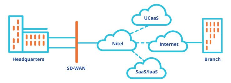
**Cisco on-ramp**, available with VMware or Cisco Advantage, actively monitors multiple paths to cloud destinations, including paths over the Nitel network, automatically routing traffic over the optimal path.
